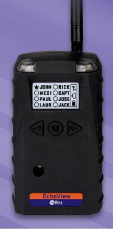
The EchoView Host is a mini-controller that creates a self-contained intelligent wireless network that supports up to 8 monitors. The easy-to-read display allows connected devices' names to be customized for easy identification of the real-time readings. The EchoView Host provides immediate remote notification of alarm conditions to keep workers informed, connected and protected.
